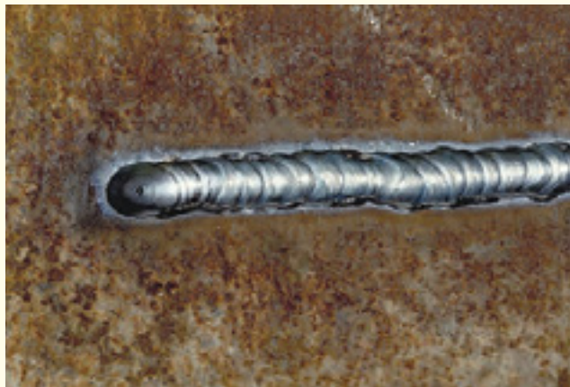
FIGURE 32-1 Gas metal arc welded (GMAW) on 16-gauge mild steel. Larry Jeffus
